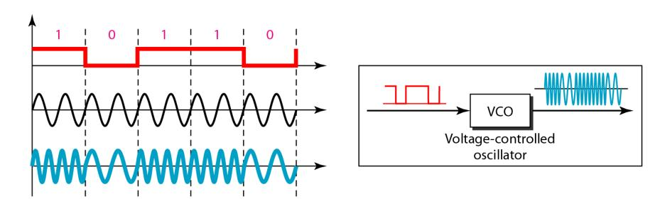
We need to send data 3 bits at a time at a bit rate of 3 Mbps. The carrier frequency is 10 MHz. Calculate the number of levels (different frequencies), the baud rate, and the bandwidth.
