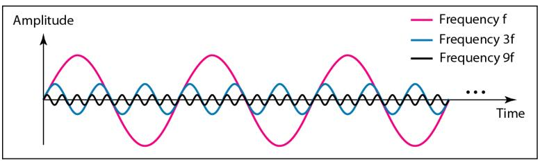
a. Time-domain decomposition of a composite signal
