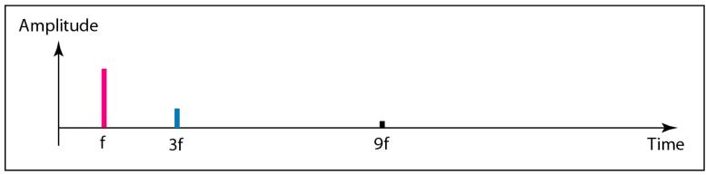
b. Frequency-domain decomposition of the composite signal
