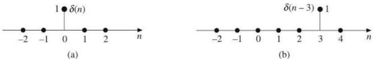
Figure 8 Discrete-time (a) Unit sample sequence, (b) Delayed unit sample sequence.
