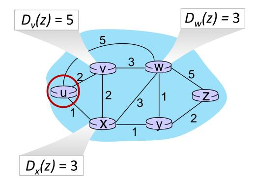
Bellman-Ford equation says:  $D_u(z) = \min \{ C_{u,v} + D_v(z), C_{u,x} + D_x(z), C_{u,w} + D_w(z) \}$  $= \min \{2 + 5, 1 + 3, 5 + 3\} = 4$
