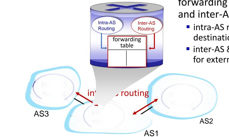
forwarding table configured by intraand inter-AS routing algorithms
